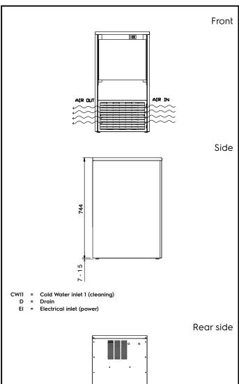
**Electric** Supply voltage: 220-240 V/1N ph/50 Hz Electrical power max: 0.25 kW Capacity: Bin capacity: 15 kg **Key Information:**
